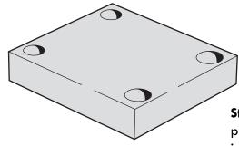
Standard Cover Plate - includes o'ring pockets on the bottom surface to provide o'ring sealing of the NFPA valve pattern. Mounting provisions include four (4) holes (6 on D08 cover plate) on the top surface of the cover plate. Mounting hardware, locating pins (w/D03 and D08 only) and viton o'ring are provided.
