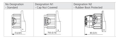
In case of solenoid malfunction or power failure, the spool of valve can be shifted with a manual override under condition that the P channel is pressurized. The main spool is operated hydraulically after shifting the control spool with the manual override. The pressure in T port does not exceed 25 bar (363 PSI). For alternative manual overrides contact our technical support.
