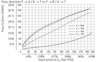
The coil current initializing the flow through the proportional directional valve can differ due to the production tolerances in a range of  $\pm$  6% of the limit current.
