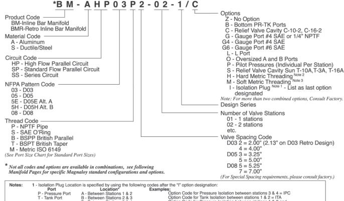
Option Code for Tank Isolation between stations 1 & 2 = ITA Option Code for Pressure Isolation between stations 1 & 2 and Tank Isolation between stations 2 & 3 = IPATB B - Between Stations 2 & 3 C - Between Stations 3 & 4
