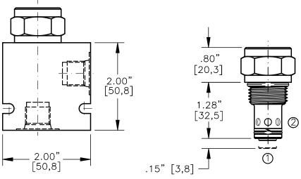
NOTE: CAVITY BOTTOM HOLE MUST ALLOW FOR POPPET EXTENSION (.570" DIA.) FOR ALUMINUM OR STEEL VALVE HOUSING CONFIGURATIONS SEE PAGE 0-012.1
