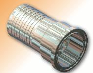
The HBS connector ingeniously permits a reliable O-R sealed junction between the inlet hose and SAE 4-Bolt pad components. Designers can have O-Ring sealing and end-to-end, from reservoir to pump inlet, even with suction hose runs.
